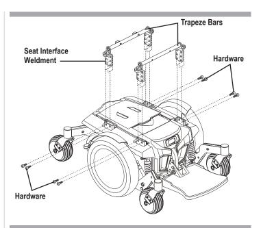
Figure 14. Seat Height/Angle Adjustment
