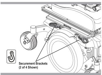
Figure 12. Transit System Securement Brackets
