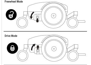
Figure 2. Manual Freewheel Lever Operation
