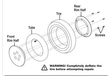
Figure 23. Drive Wheel Disassembled
