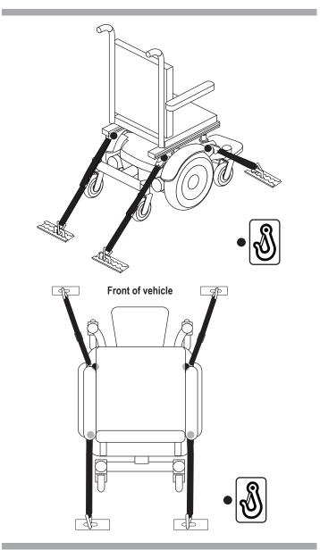
Figure 13. Unoccupied Transit System Securement Points
