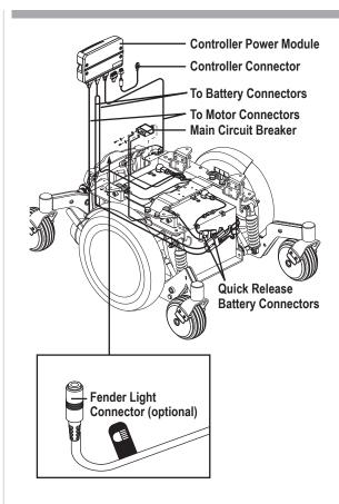
Figure 1. Electrical Components
