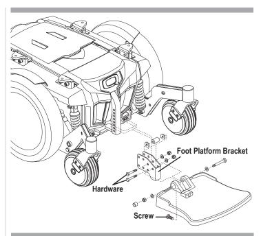
Figure 17. Foot Platform Adjustment
