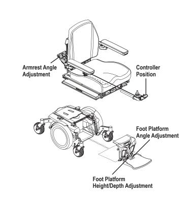
Figure 5. Assembly View
