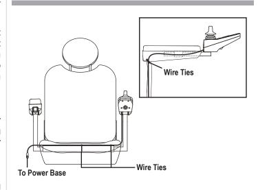
Figure 8. Controller Harness Routing on a Contour Seat
