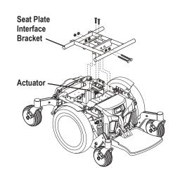
Figure 11. Power Elevating Seat Actuator
