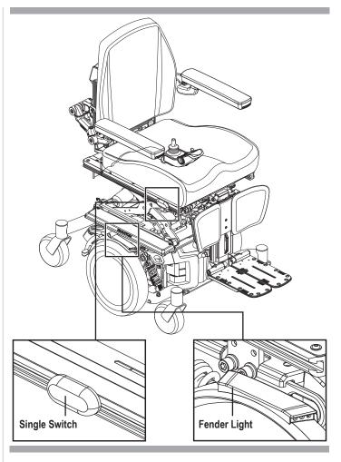
Figure 4. Single Switch to Operate Fender Lights
