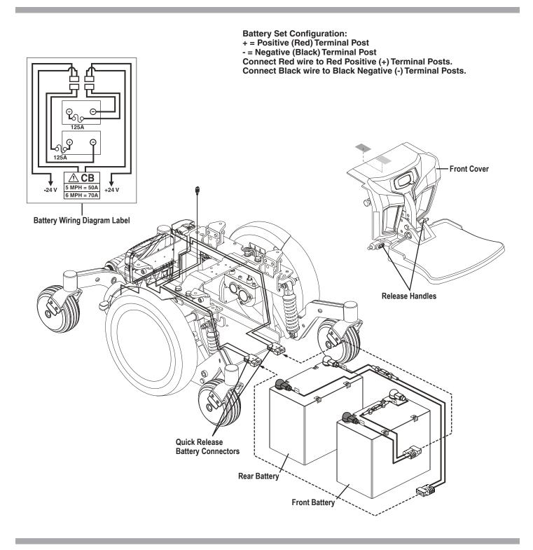
Figure 24. Battery Installation
