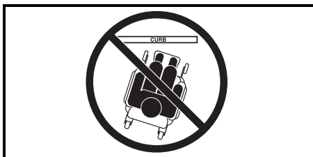
Figure 3. Incorrect Curb Approach
